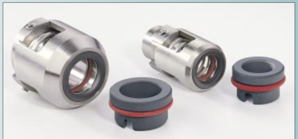
Balanced seal type 82EH for high pressure, bi-directional, all metal parts in titanium with SiC faces.
